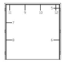
7. Check the door and frame alignments again. If they are all still ok, open both doors and fit the remaining frame fixings in the sequence shown. If not, remove some fixings and start again at Step 3.
