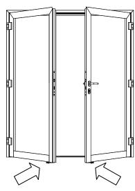
4. Open both doors carefully to approx. 45°, taking care not to disturb the frame, then temporarily pack the lock edges of the door leaves off the floor, keeping the jambs vertical.
