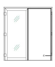
**6.** Close and bolt the fixed leaf, then with the active leaf nearly closed, check the alignment between the meeting stiles for an even seal gap, at both the top and bottom of the doors.
