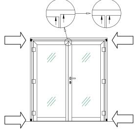
2. Align and wedge the frame into the opening, using temporary packers at the corners.
