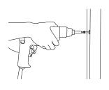
**5a.** First fix in the sequence shown, with 2 fixings in the fixed leaf jamb and 1 in the active leaf jamb.
